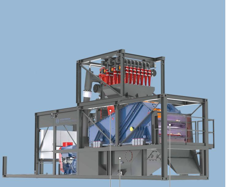
Hydrocyclone AT 66-500 Multi chamber underflow sump 1640 II Hybrid Double deck screening machine
